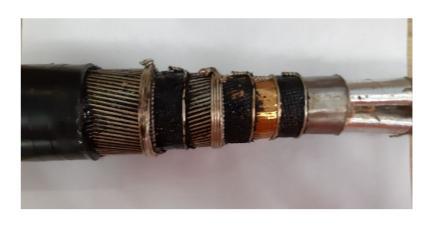
11kV 3C Cable 1967 Power Cables Australia
