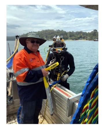
Submersible detector coil used by Coastal Cable Locators to find 132kV cables, DCL certified, NULCA member
