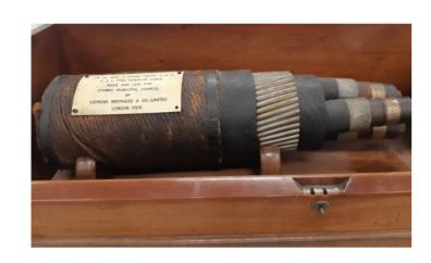
33kV HSL Cable 1928 Siemens
