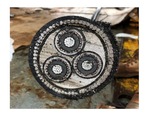
11kV 3C Cable 2010 (3C overall lead sheath)
