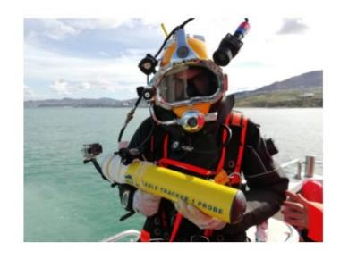
Fully Submersible Cable Locator used by McLennan's Diving to locate 11kV cables
